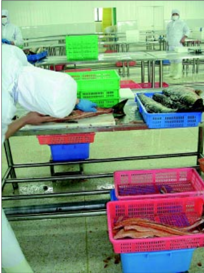
Station 1. Filleting dressed (headed and gutted) salmon. Fish are cut in half lengthwise and the vertebrae removed.
