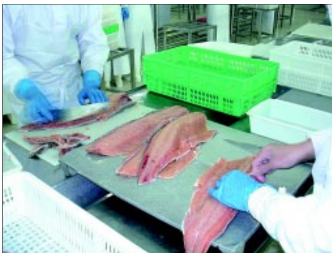
Station 2. Fillet trimming and pin bone removal. Pin bone removal is done with the use of tweezers.
