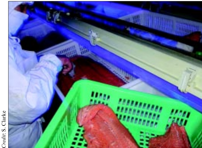
Station 4. Parasite removal under ultraviolet (UV) light. About 20 people were working with tweezers to remove parasites visible from the surface, mostly in the belly area. UV light is necessary to spot parasites when working with salmon. Chum are said to have a particularly high number of parasites.
